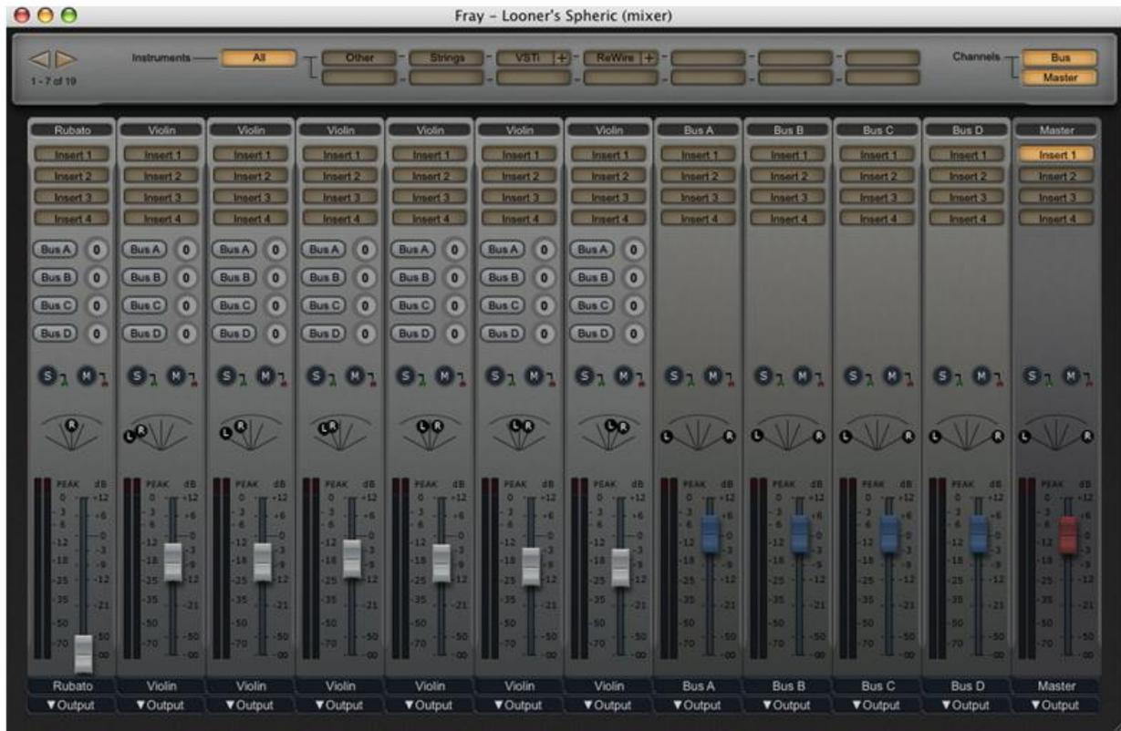
This is the mixing board of the same work. Each staff has its own mixer track. There are four inserts per track and four busses. Each fader has its own Peak Meter and dB calibration. Of course, there's panning, mute and solo.
