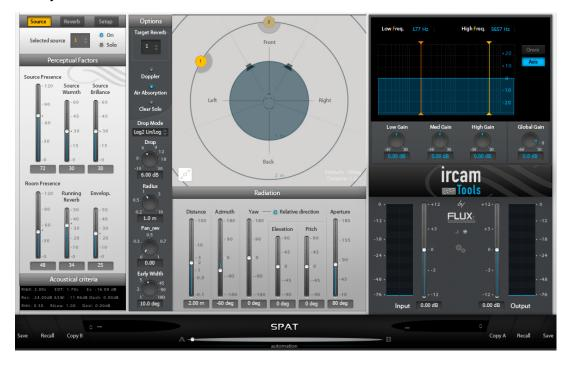
The Display, pictured below in Day view, is where you can manually spatially place and set stereo width. This is a much easier graphic to work with then the previous version. In stereo, the 1 is left and 2 is right.
